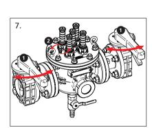
7. Re-open both isolation valves then refill the system as required. Bleed the air from the filter using the air vent. Ensure all magnets and pockets remain dry at all times. Remove any excess fluid from the
