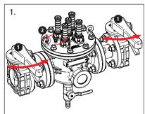
1. Check the MagnaClean sight glass for build-up of black iron oxide. Turn off the boiler and isolate the electrical supply prior to servicing. Turn off the open the air vent located on top.
