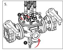
5 Close the inlet isolation valve once the water runs clear, then close the drain point by turning off the drain valve or replacing the drain plug. Close the
