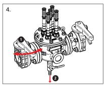
4. Partially open the inlet isolation valve, leaving the outlet isolation valve in the closed position and allow the deposits to drain through.
