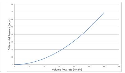
3" MagnaClean Pressure Differential vs Flow Rate
