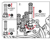
and hold the grey locking ring, then carefully pull up the magnet. After the magnet is released, hold down the locking ring and continue to slowly lift the magnet assembly until it locks into the service position. Ensure that the magnets are not removed
