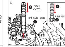
6. To replace the magnets to operational mode, lift and hold the grey locking ring up and slowly push the magnet assembly down. Release the locking ring and continue to slowly push down the magnet assembly until it locks into operational mode. Repeat the procedure for each magnet assembly.
