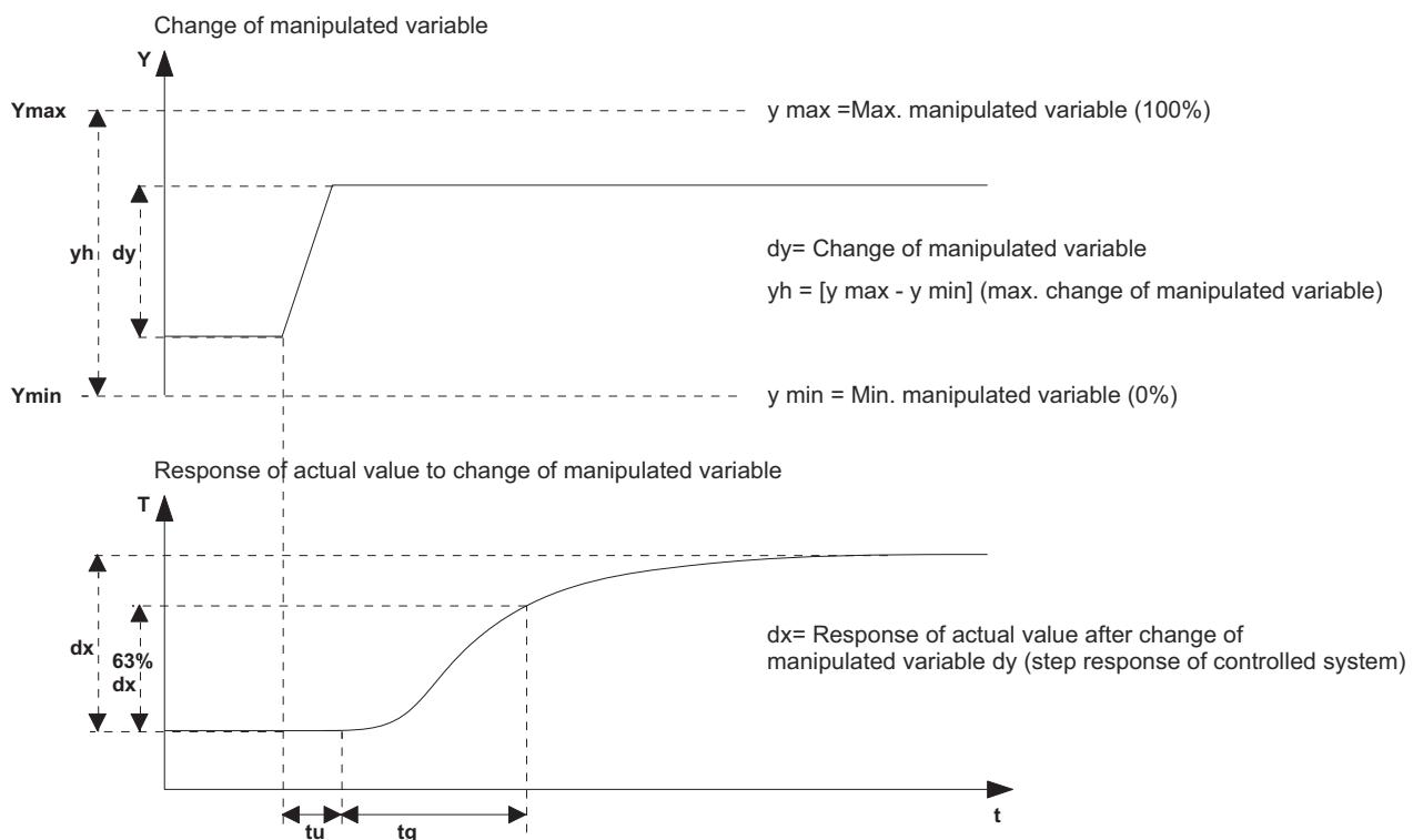
$$\text{P-band } X_p: X_p = 1.5 * (t_u/t_g) * y_h * dx / dy$$
